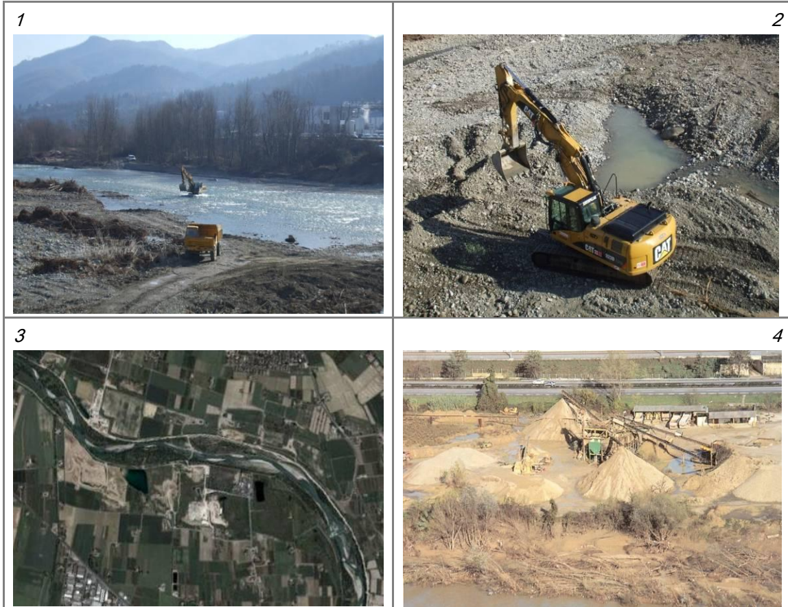
Figure 68 Sediment removal. (1) and (2) Recent and current activity; (3) and (4) indirect indicators of past activity are the presence of mining sites. In the case of partly- and unconfined channels, Class B1, B2 or C depends on the occurrence of sediment removal in the past (since 1950's) and/or in recent times (last 20 years).
