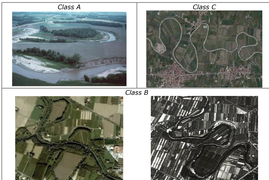
Figure 30 Presence of typical fluvial forms in the floodplain. Class A : meandering river with a recent cut-off. Class C : meandering river with complete absence of landforms in the plain. Class B : traces of abandoned meanders exits (photo on the left), disconnected from the channel because of bed incision. The observation of the aerial photos of the 1950's (photo on right) enables verification that these forms have been abandoned during the last decades.
