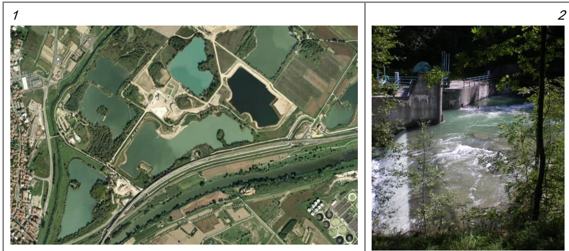
Figure 51 Other structures (besides those defined for A1) that can cause an alteration of flows within a reach. (1) Retention basins; (2) discharge abstraction.
