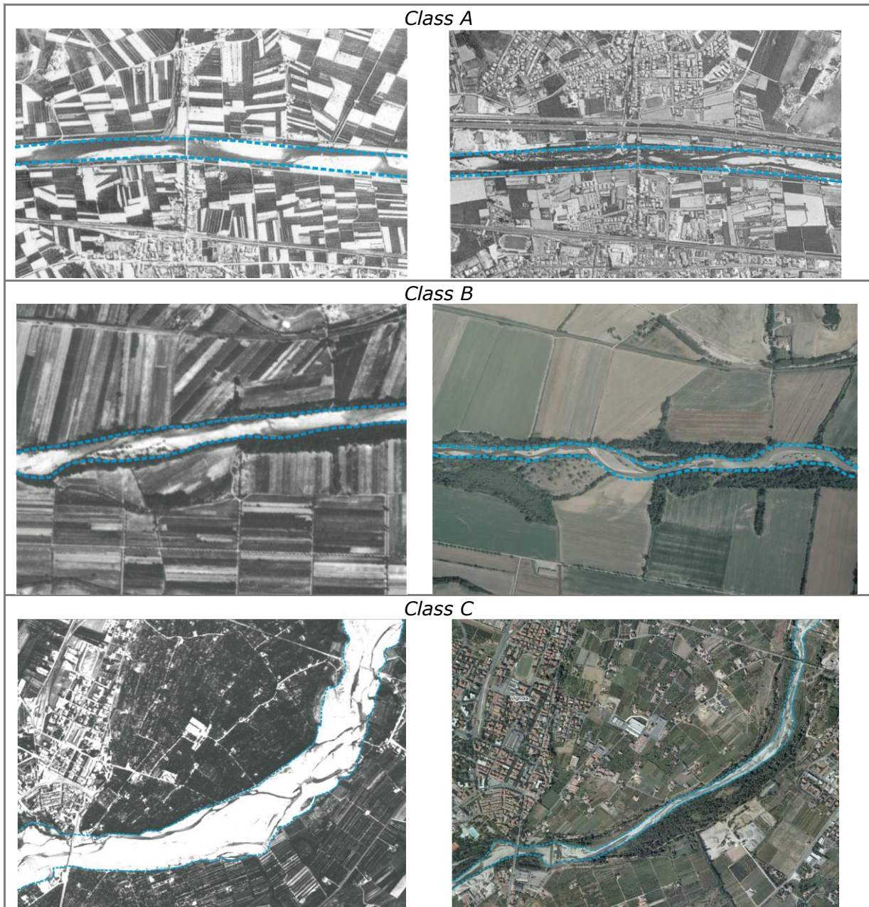
Figure 72 Adjustments in channel width (on the left aerial photo dated 1954, on the right the current situation). Class A : very limited channel narrowing (< 15%). Class B : channel narrowing from 15% to 35% of channel width in 1930s-60s. Class C : very intense channel narrowing (> 35%).
